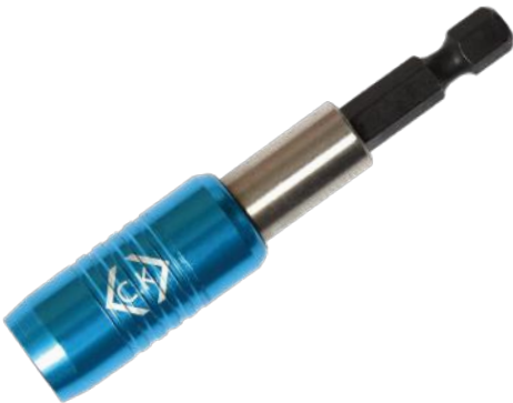
Screwdriver Bit Holder Screw Grip Magnetic base retains the bit in place. Magnetic collar holds the screw in place. 6.35 Hex.
