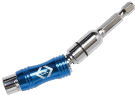
Screwdriver Bit Holder Pivot Joint Magnetic base securely retains the bit in place. Pivoting head for when straight line access isn't possible. Lockable collar for use as a straight bit holder. 6.35 Hex.
